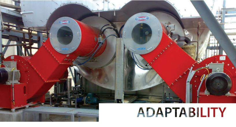
Combustion air is delivered via a remote or directly mounted centrifugal fan. The fan has a direct coupled, backward curved impeller, and can be supplied with a flange mounted silencer. The air damper blades are operated using fully enclosed bearing assemblies, this allows hysteresis free operation with infinite repeatability.
