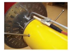
The unique spider head assembly offers the user high turn down ratios. It was initially designed to be fired when using fuels with high burning velocities such as Propane or Hydrogen. Unlike the split head, the fuel is introduced after the diffuser plate enabling the flame to establish good retention whilst maintaining excellent mixing. Limpsfield will design and engineer the correct solution to suit your application.
